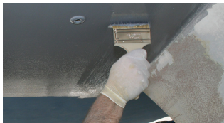
Lay off Gel Protect in opposite direction with brush
