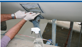
Wet scrape to remove old antifouling
