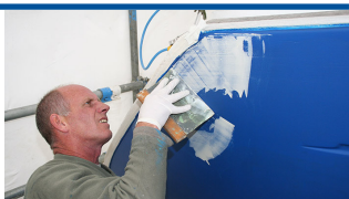
Fairing any defects
