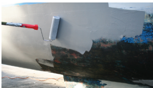
Apply Underwater Primer onto prepared surface
