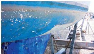
Paint blisters and lifts
